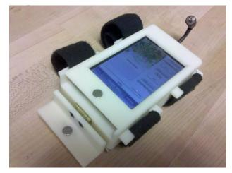
Fig. 17.8. The supervisor programs the day's schedule using an intuitive iPod Touch application.
